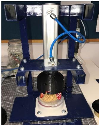
The photographs show the accuracy with which the reproduction occurred. The bottom photo involves a prototype test rig that was quickly fabricated for Ingenia and fitted with a pneumatic ram to reproduce the coupling actions with the exact dimensions and clearances of the equipment on the factory floor. This was presented as a desktop presentation of a fully functioning prototype coupling in the client's boardroom.
